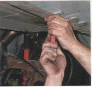
With the suspension and exhaust out of the way, the heat shield for the gas tank is unscrewed and the tank is ready to come out.
