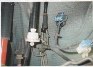
But first, the fuel line must be unplugged at the filter, the return line must also be disconnected, the plug for the gas tank removed, and finally, the evap tube for the tank with a set of pliers.
