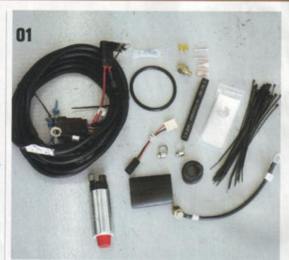
The Racetronix LU305 kit comes with a high-performance Walbro fuel pump and everything you need for the installation. Racetronix also includes a plug-and-play auxiliary relay and harness assembly complete with Delphi Weatherpack connectors. This assembly ensures that the pump has a constant 13.5 volts supplied to pump at all times for maximum fuel output.
